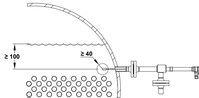
Remark: Provide a spacing of at least 40 mm between the probe central electrode pole and any metallic parts such as the boiler wall, tubes and other metallic fittings. The probe must be installed in such a way that it is always in contact with water and wetted parts fully immersed, without air gaps. As far from the feedwater inlet as possible and away from the steam bubbles, at least 100 mm below the boiler low water level.
