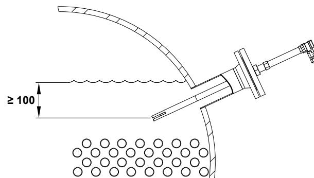
Remark: Installation at a 45° angle, only possible when probe is fitted with a threaded outer shroud.
