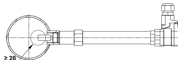
Remark: Probe can be fitted onto a "T" connection or onto the F2132 sensor chamber, providing that it is always in contact with water and wetted parts fully immersed, without air gaps. Any metallic parts near the probe must be at a minimum distance of 20 mm from the central electrode pole. Ensure the connection on the boiler is safely below the boiler low water level.
